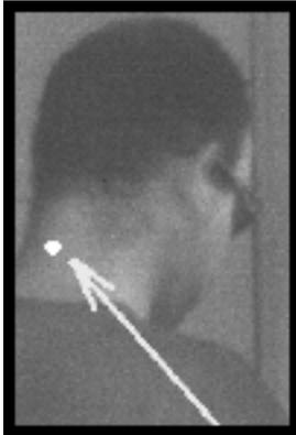
Unlike classic laser beam eavesdropping, the new method does not rely on interferometer or a reflecting diaphragm, like a window. A single laser beam is aimed at the object to be monitored (a person and a cell phone were used in these tests).
